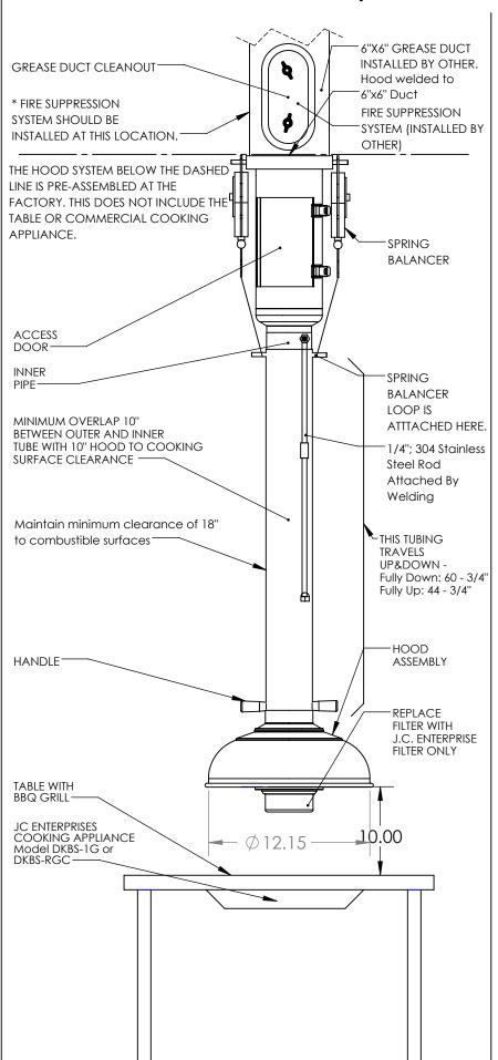
Model No. DKBHS is designed for exhaust air applications and to use it with UL listed blower (fan) assemblies.
